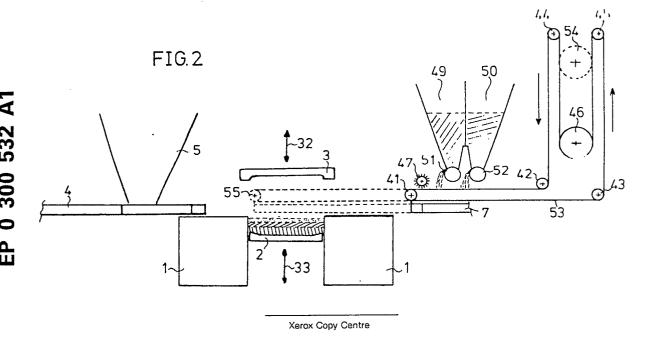
Ceramic flooring tile, set of mutually distinguishable flooring tiles, method for producing a set of flooring tiles and device for carrying out said method.
