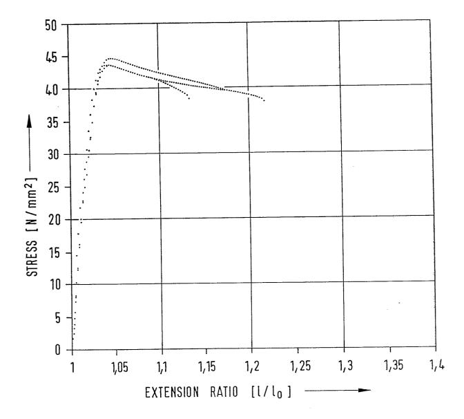
FIG. 4, stress/strain behaviour of starch processed according to Example 2: residence time: 750 seconds; screw speed 100 rpm; break strain: 8,8± 3.1 % break stress: 33,8± 7.7 MPa: break energy/unit area 108± 4.4 kJm<sup>-2</sup>.
