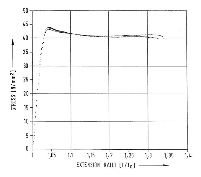
FIG. 2, stress/strain behaviour of starch, processed as described in Example 1(b): residence time: 450 seconds; screw speed 125 rpm; break strain: 29,4 ± 2.0 %; break stress: 39,3 ± 0.2 MPa; break energy/unit area: 401 ± 30.6 kJ m<sup>-2</sup>.
