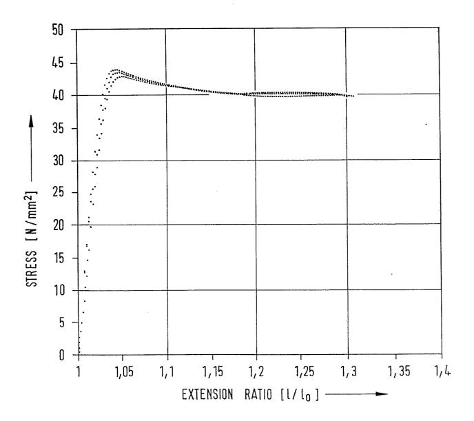
FIG. 3, stress/strain behaviour of starch processed according to Example 2: residence time 750 seconds; screw speed: 75 rpm; break strain:  $18,0 \pm 4.7$  %; break stress:  $33,8 \pm 7.7$  MPa; break energy/unit area:  $242 \pm 68$  kJ m<sup>-2</sup>.
