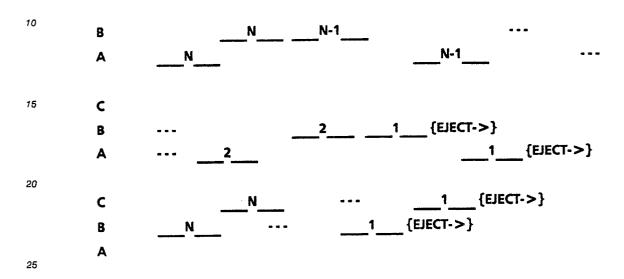
In this above description the bins are referred to as A, B and C, rather than 112, 114, and 116, in order to emphasize that the sequence is not limited to that physical order. Each bin has its own integral gate, solenoid-operable in any order programmed by the controller. Since the gates move with their bins, the maintain interdigitation with the transport 110 belts, sheets can be loaded into bins in any bin position, and while the bins are moving.
