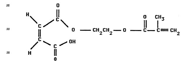
Care must be taken during the heating process above to keep the reaction process at or below about 80-90 degrees C to avoid premature polymerization due to the methacrylate group.
