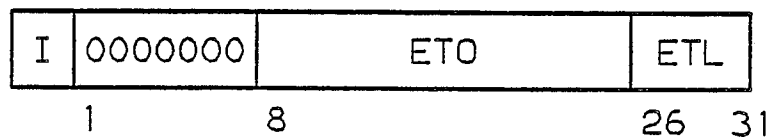
FIG.7 LINKAGE-TABLE ENTRY (LTE)
