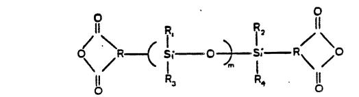
wherein R is substituted or unsubstituted aliphatic trifunctional radicals of 1 to 12 carbon atoms or substituted or unsubstituted aromatic trifunctional radicals of 6 to 10 carbon atoms, and wherein one or
