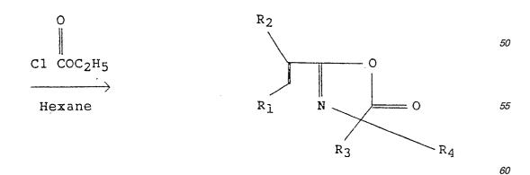
The first step being a Shotten-Bauman acylation of an amino acid. The polymerizable functionality is introduced by using either acryloyl or methacryloyl chloride. The second step involves a ring closure with a chloroformate to yield the desired oxazalone. The product is isolated and purified by the usual procedures of organic chemistry.
