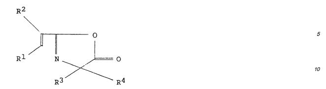
where  $R^1$  and  $R^2$  independently denote a hydrogen atom or a lower alkyl radical with one to six carbon atoms, and  $R^3$  and  $R^4$  independently denote alkyl radicals with one to six carbon atoms or a cycloalkyl radical with 5 or 6 carbon atoms.
