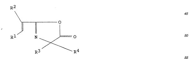
where  $R^1$  and  $R^2$  independently denote a hydrogen atom or a lower alkyl radical with one to six carbon atoms, and  $R^3$  and  $R^4$  independently denote alkyl radicals with one to six carbon atoms or a cyclohexyl radical.
