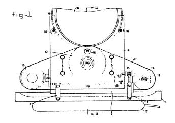
Device for grinding a bearing journal of the crankshaft of a combustion engine, in particular a diesel engine.
