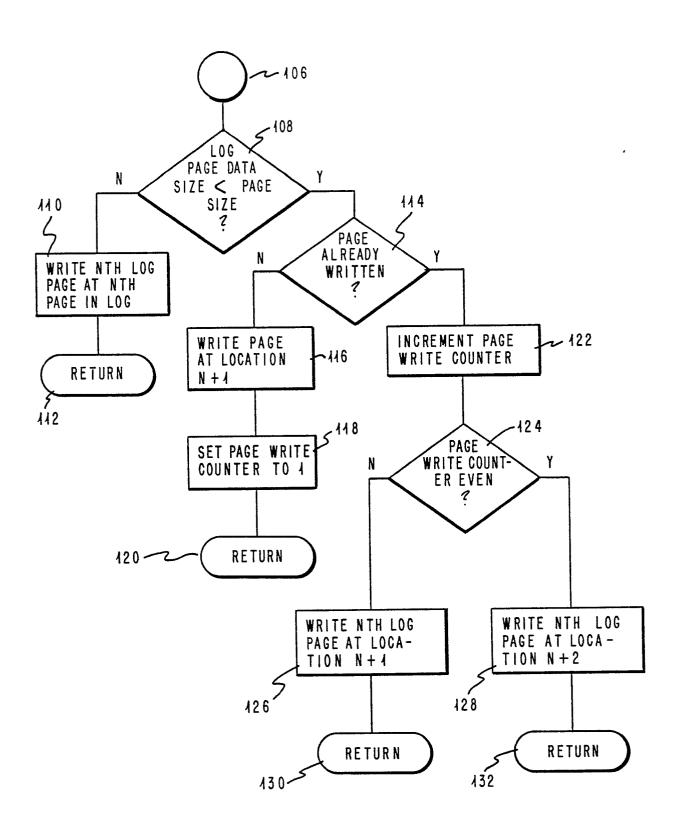
FIG. 6 FORWARD PROCESSING (NORMAL)
