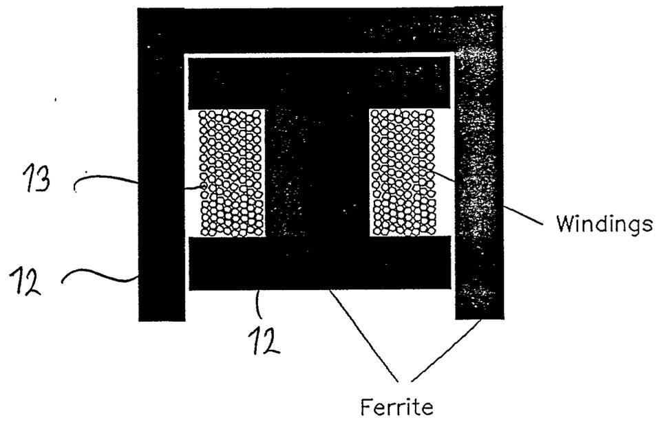
Figure 3 Typical Inductor Constuction
