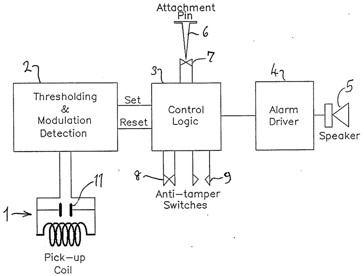
Figure 1. Block Diagram of Active Tag
