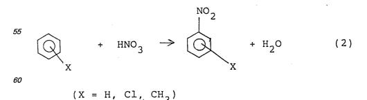
According to the present invention, nitrobenzenes are produced by nitration of benzenes in vapor phase with nitric acid wherein (A) acidic sheet clay minerals which are ion-exchanged with polyvalent metal ions or (B) acidic composite oxides comprising oxides of elements of the Group IVA of the Mendeleefs' periodic table and tungsten oxide, molybdenum oxide, niobium oxide or zinc oxide are used as a catalyst. . .
