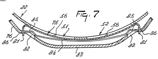
This invention relates to a spreader having a spreading member and a discharge member, the latter having at least one discharge aperture through which material can be delivered to the spreading member, a dosing slide being mounted on a bracket which is movably coupled to the discharge member, said dosing slide being adjustable along the discharge aperture to open or close the aperture to a lesser or greater extent.
