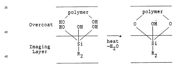
A useful hydrolyzed polyoxysilane in the imaging layer does not adversely flow, smear or distort the imaging layer or a contiguous layer, such as an overcoat layer, at processing temperature, typically within the range of 100°C. to 200°C.
