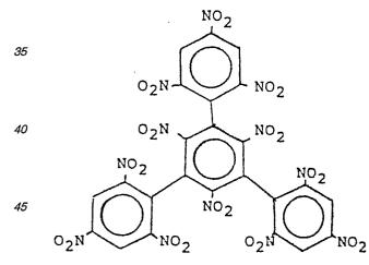
50 It is a secondary explosive with good thermal stability and high initiation sensitivity. One of its immediate applications, although its use is not limited to this, is as a detonator. Such detonators typically take the form of booster cups or EBW detonators. Both these devices are used in oil well perforation.
