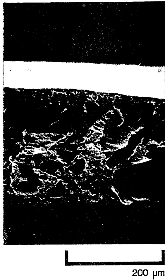
Figure 38. Example 43. SEM of a Cross Section of an Asymmetric-Membrane Capsule Wall Made With a Blend of Ethylcellulose and Cellulose Acetate Phthalate. 4.5 cm = 200 μm.
