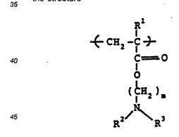
wherein m can be 1 or 2, R<sup>1</sup> represents hydrogen or -CH<sub>3</sub>, R<sup>2</sup> represents hydrogen or an alkyl group having up to 10 carbon atoms, and R<sup>3</sup> represents an alkyl group having up to 10 carbon atoms;
