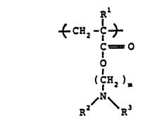
wherein m can be 1 or 2,  $R^1$  represents hydrogen or -CH<sub>3</sub>,  $R^2$  represents hydrogen or an alkyl group having up to 10 carbon atoms, preferably 1 to 4 carbon atoms, and  $R^3$  represents an alkyl group having up to 10 carbon atoms, preferably 1 to 4 carbon atoms;
