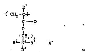
wherein p can be 1 or 2,  $R^1$ ,  $R^2$ , and  $R^3$  are as defined above,  $R^4$  represents an alkyl group having up to 10 carbon atoms, and X<sup>-</sup> represents a halide ion,  $R^2SO_4^-$ ,  $R^3SO_4^-$  or  $R^4SO_4^-$ ;
