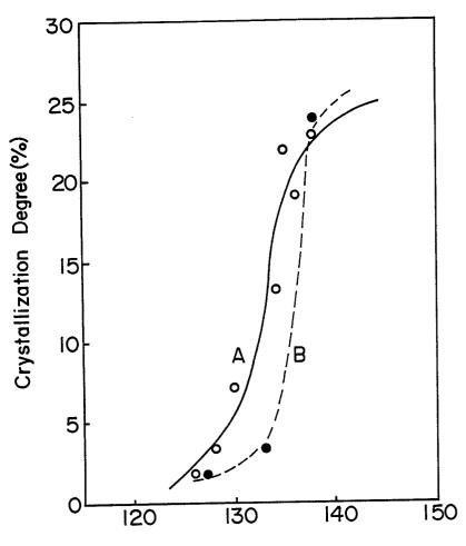
Temperature of Casting Roll (°C)
