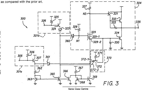
This invention pertains to electronic circuits, and more particularly to a sense amplifer for sensing low level signals and providing higher level output signals. The teaching of this invention is particularly useful in sense amplifiers for use with programmable logic devices.
