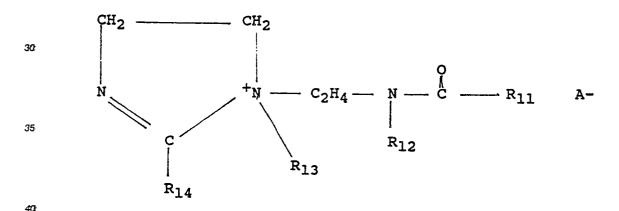
wherein  $R_{13}$  is a hydrocarbyl group containing from 1 to 4, preferably 1 or 2 carbon atoms,  $R_{11}$  is a hydrocarbyl group containing from 8 to 25 carbon atoms,  $R_{14}$  is an hydrocarbyl group containing from 8 to 25 carbon atoms and  $R_{12}$  is hydrogen or a hydrocarbyl containing from 1 to 4 carbon atoms and  $A^-$  is an anion, preferably a halide, methosulphate or ethosulphate.
