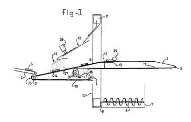
The present invention relates to a method for forming a moving, continuous bed which is composed of granular and/or pulverulent flowable material and which is of constant thickness. Such a method is known from NL-A-7810080. In said known method, the material is deposited on the belt from a feedstock container and is more uniformly distributed by means of a pressure roller.
