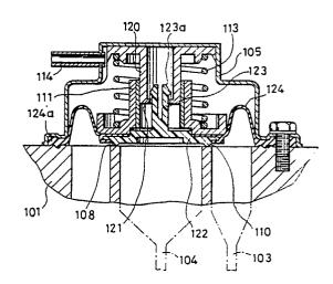
Supercharged pressure control valve apparatus
