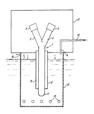
Device for measuring the refractive index of a fluid, in particular intended for measuring the density of that fluid or the concentration of a substance dissolved in that fluid.
