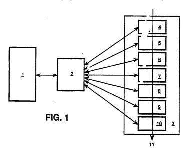
The invention relates to a method of preparing an item to be mailed using a printer in which a main document is printed and a line of mail preparation stations comprising an inserter station, responsive to an output comprising instructions for controlling the printer and the mail preparation stations said instructions for controlling the mail preparation stations being detected and fed to those mail preparation stations.
