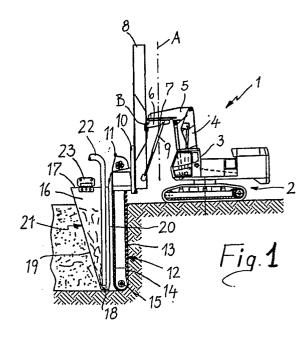
The object of the present invention is a method for executing monolithic continuous straight or circular structural walls and an equipment for realizing said method.
