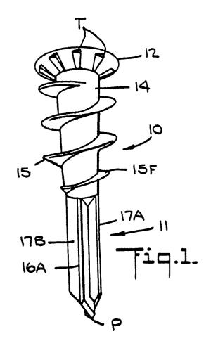
SELF-DRILLING WALL ANCHOR
