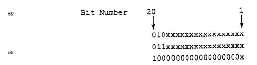
The first eighteen bits of the multiplier go through the modified Booth recoding process in modified
