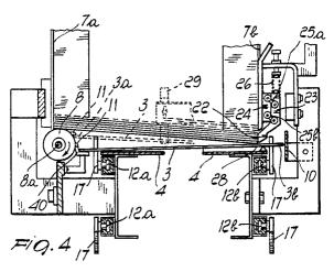
The present invention relates to an automatic device for feeding strips or the like to a conveyor element, in particular for machines for assembling packing boxes, such as for example fruit trays or the like.
