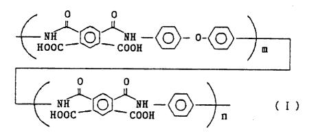
followed by the imidization thereof, the amount of said tertiary amino compound added to the solution being 10 to 50 parts by weight per 100 parts by weight of solid polyamic acid contained in said resin solution. According to the present invention, a flexible printed circuit board which is free from curling, wrinkling and warping, and which has excellent heat resistance, electrical characteristics and mechanical properties is provided with a simplified production process.
