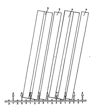
"STORALL CD FLAP" IS A STORAGE SYSTEM FOR COMPACT-DISCS (CD'S), BOTH DOUBLE AND SINGLE CD'S, INDIVIDUAL PACKED IN STANDARD PACKAGINGS. STORED WITHIN THIS SYSTEM, CD'S CAN BE TILTED TO AND FRO, WHILE THEY REMAIN IN AN OBLIQUE PARALLEL POSITION AFTER THE OPERATION. DOUBLE AND SINGLE CD' SCAN BE STORED IN ANY ARBITRARY ORDER WITHOUT LEAVE A BLANK.
