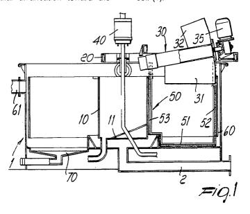
The present invention relates to an apparatus for continuous purification of liquids, and in particular to an apparatus for the continuous clarifying of liquids with suspended solid substances by means of the dissolved gas flotation process.
