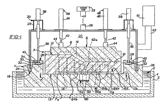
This invention relates to an improved apparatus and method for the differential pressure, countergravity casting of a melt in such a manner as to pass the melt through a reaction chamber to selectively introduce alloyant into the melt as it is countergravity cast into the mold.
