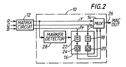
This invention relates to the encoding and decoding of multiplexed analog components (MAC) video signals.
