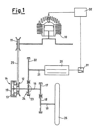
This invention relates to a hybrid propulsion system for vehicles, in particular for road vehicles.
