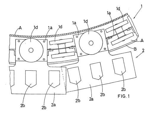
This patent application concerns a flexible segmented belt for use as a pulling, guiding and transport element in automatic overhead conveyor systems.
