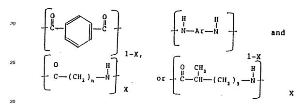
where n is 4 or 5; X is from 0.01 to 0.50 and Ar is a radical selected from 3,4'-oxydiphenylene, 4,4'-oxydiphenylene, 4,4'-sulfonyldiphenylene, 1,3-phenylene and mixtures of such radicals with each other or mixtures of such radicals with up to 50 mol percent of 1,4-phenylene radicals based on the mixture of radials.
