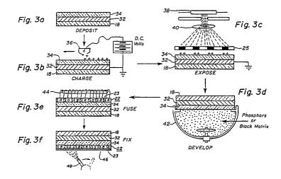
The present invention relates to a method of electrophotographically manufacturing a luminescent screen assembly and, more particularly, to a method in which an improved plasticizer is utilized with a photoconductive layer to minimize the cracking of the layer.
