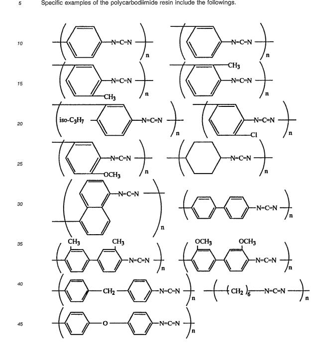
In the above formulas, n is a degree of polymerization and is in the range of 10-10,000, preferably in the range of 50-5,000. 50
