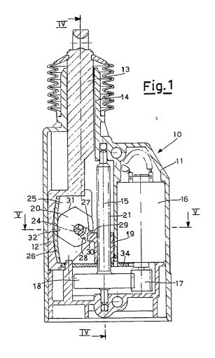
The present invention relates to an improved arrangement for actuating motor vehicle door locks whereby, a closure of one of the locks generally at the front, is automatically accompanied by a closure of all other locks.
