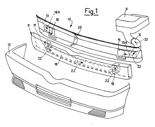
This invention relates to an air intake for engine feed.
