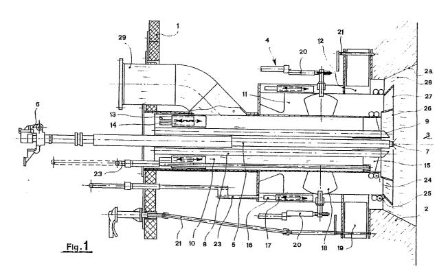
The present invention relates to an improved burner for fuel oil and fuel gas with low NOx production.
