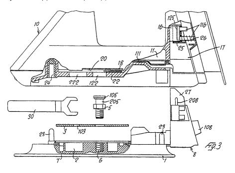
The invention relates to a steam iron, particularly of the so-called "drop type", wherein in order to cause an instantaneous steam production, the water which is contained in a reservoir incorporated in the iron falls drop-by-drop into a vaporization chamber provided in the inner side of the sole plate of the iron, in registry with the heating resistance of said sole plate, the so-generated steam being conveyed outwards through a plurality of holes in the sole plate.
