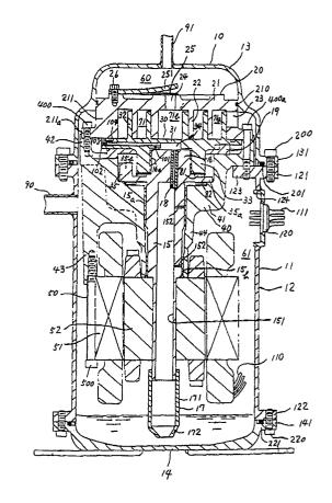
This invention relates to a hermetically sealed scroll type refrigerant compressor, and more particularly to a lubricating mechanism thereof.
