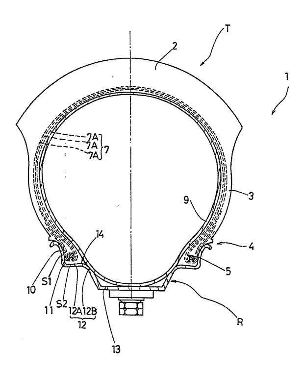
The present invention relates to a motorcycle tyre and rim assembly capable of preventing a tyre from coming off its rim effectively even when the internal pressure is lowered during travel due to a flat tyre or the like, and hence enhancing the safety of travel.
