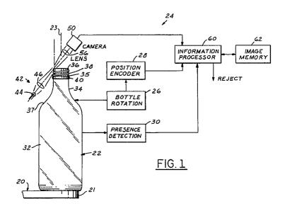
The present invention is directed to optical inspection of translucent containers, and more specifically to an apparatus and method for inspecting the finish of containers for vertical checks.
