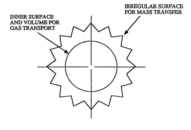
MASS TRANSFER TUBING (cross section)
