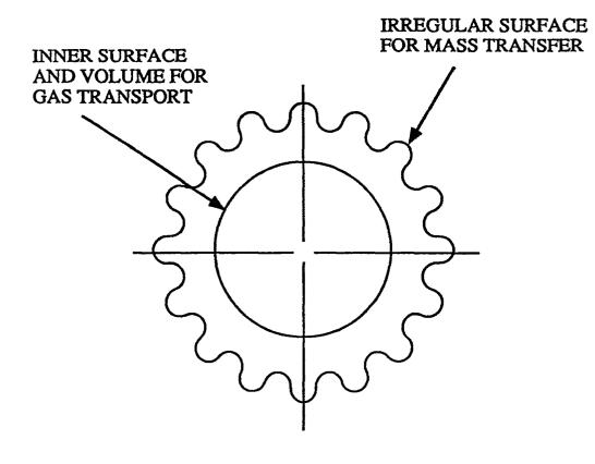
MASS TRANSFER TUBING (cross section)
