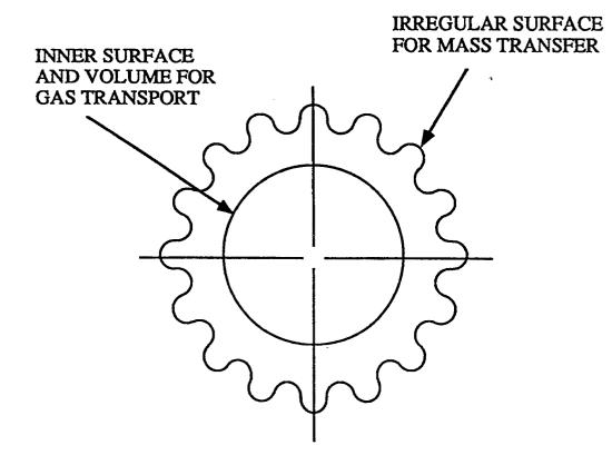
MASS TRANSFER TUBING (cross section)
