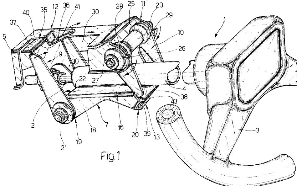
The present invention relates to a collapsible energy absorbing system for supporting a steering column of a vehicle, capable of preventing or at least containing possible injuries to the driver of the vehicle in the event of impact during an accident.
