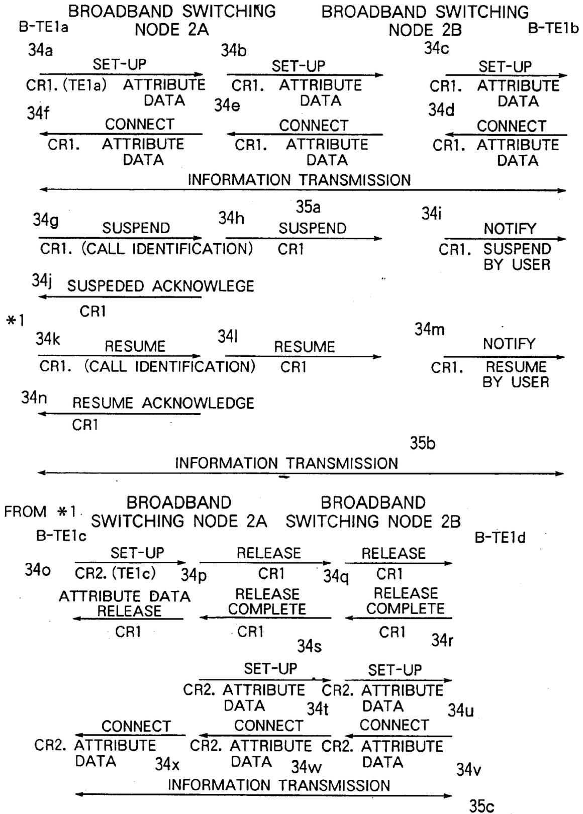
ALTHOUGH VALUE OF CR IS LOCAL VALUE CLOSED IN INTERFACE, IT IS TREATED AS SAME VALUE FROM END TO END FOR SIMPLICITY.
