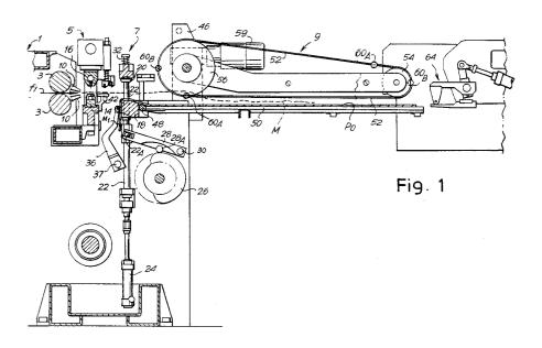
The invention relates to a device for the accumulation of bags made of thermoplastic film or similar manufactured articles in order to form them into a uniform stack during their production, comprising welding and cutting bars. The abovementioned device makes it possible to carry out the formation of the stack uniformly and rapidly and without any damage to the manufactured articles which are gradually stacked.
