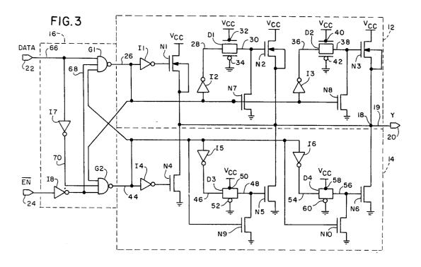
This invention relates generally to semiconductor integrated circuits and more particularly, it relates to a CMOS output buffer circuit which has a significant reduction in ground bounce.
