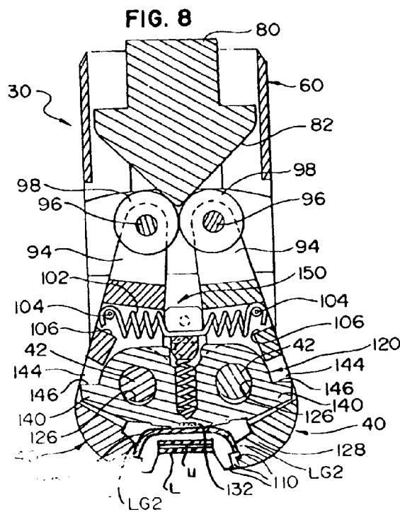
This invention relates to securement of the overlapping ends of a tensioned strap loop around a package or other object. More particularly, the present invention relates to an improved method and mechanism for crimping a seal around the overlapping lengths of strap to hold the strap lengths together.
